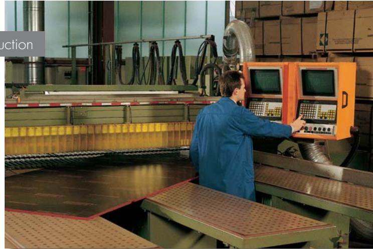
Frame elements are cut to size on a special-purpose CNC-machine. While still clamped in place the elements are mitered and the weld is prepared.
